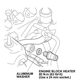
12. Plug the heater harness connector into the engine block heater. Make sure the heater harness connector is fully seated.
