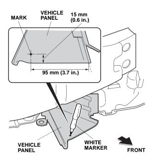
21. Using a pushpin, pierce the mark on the vehicle panel.
