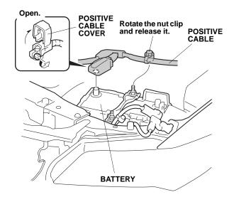
7. Remove the battery (two nuts and the battery plate) Remove the battery upper cover, and battery under cover).
