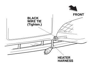
30. Attach the protective cap to the front bumper, and plug the heater harness connector into the protective cap.
