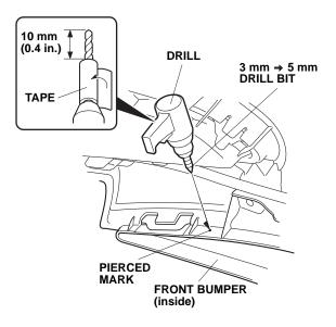
28. With the help of an assistant, bring the front bumper close to the vehicle. Attach the heater harness to the drilled hole in the front bumper with one loosely-installed black wire tie, then reinstall the front bumper.
