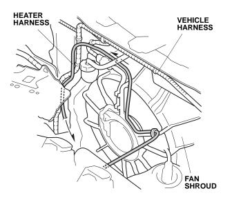
16. Using two black wire ties and three white wire ties, secure the heater harness to the fan shroud ribs and the vehicle harness.
