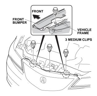
• Remove 2 self-tapping screws, 2 bolts, 2 short clips, and 12 medium clips.
