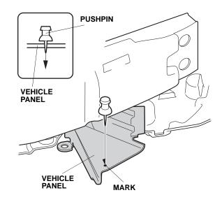
22. While wearing eye protection, drill the pierced mark with a 3 mm drill bit, then enlarge the hole with a 5 mm drill bit. Remove any burrs.
