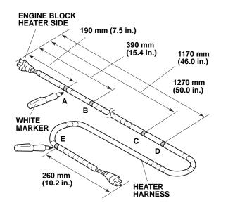
9. Install two wire ties with clips to the heater harness at points C and D.
