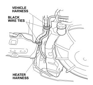
19. Route the heater harness as shown. Secure the two clips (points C and D) on the heater harness to the vehicle panel.
