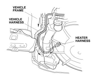
18. Using two black wire ties, secure the heater harness to the vehicle harness.
