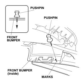
27. While wearing eye protection, drill the pierced mark with a 3 mm drill bit, then enlarge the hole with a 5 mm drill bit. Remove any burrs. To prevent drilling through the outer panel, wrap tape around the drill bit 10 mm (0.4 in.) away from the tip, or use a drill stop.
