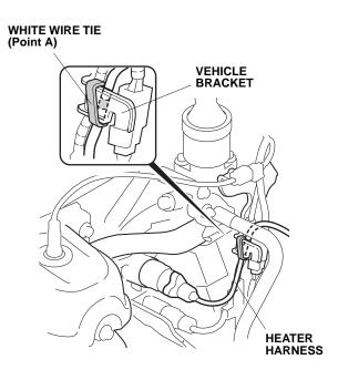
14. Route the heater harness as shown. Secure the heater harness to the fan shroud rib with one white wire tie at the white mark (point B).
